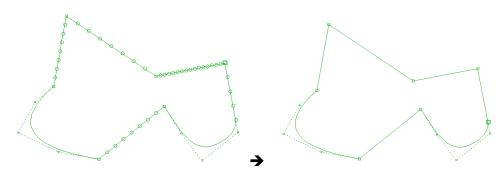
All intermediate aligned points between two ends will be erased according to a tolerance. Very useful after a vectorial import whose curves are all segmented. The goal is to minimize the number of points for machining or 3D construction.
